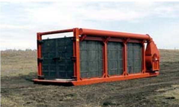
Air curtain incinerator
